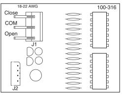
Figure-2 Typical Wiring of Three-Wire Floating Non-Spring Return Valves with Time-Out.
