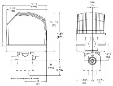
Figure-11 Modulating Spring Return Valve.
