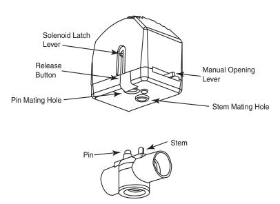
Figure-9 Three-Way Spring Return Valves.
