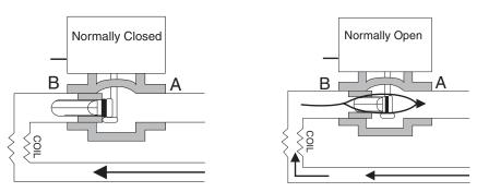
Figure-7 Two-Way Spring Return Valves.
