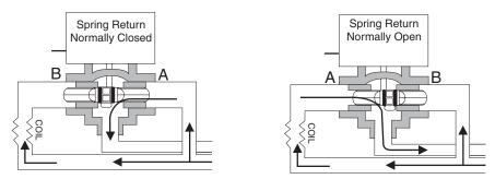
Figure-8 Three-Way Spring Return Valves.
